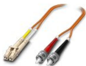
Multi-mode OM2 duplex jumper, LC-ST, UPC polishing, length 5 m
