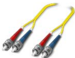
Single-mode OS2 duplex jumper, ST-ST, UPC polishing, length 2 m
