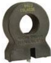
CSLA Series linear current sensor, 400 A sensed current, sink or source output, through-hole, operates on AC or DC current, bottom mount
