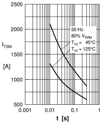
Fig. 1 Surge overload current  $I_{TSM}$ ,
