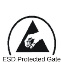
ESD Protected Gate
