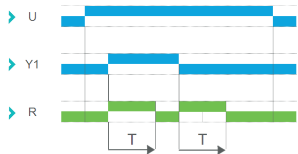
Function D - Flasher (Symmetrical) – OFF Start
