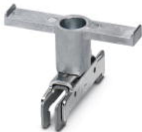
Support bracket, Bracket for busbars, set every 20 cm, length: 50 mm, width: 56 mm, height: 33.7 mm, number of positions: 2, color: silver
