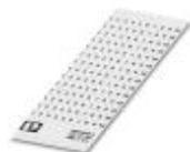
Marker card, Card, white, labeled, Horizontal: consecutive numbers 1 ... 10, 11 ... 20, etc. up to 91 ... 99, mounting type: adhesive, for terminal block width: 2.54 mm, lettering field size: 2.54 x 2.8 mm
