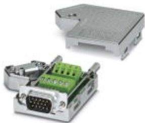
D-SUB connector, 15-pos. HD (High Density), male, one cable entry <35°, universal type for all systems, pin assignment: 1, 2, 3, 6, 7, 8, 10, 13, 14 to screw connection terminal block
