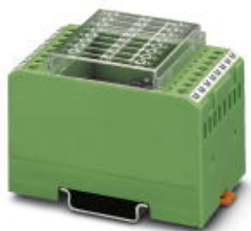
Diode module, with eight diodes, common anode, diode type 1N 5408
