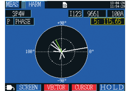
Harmonic power phase angle graph screen
