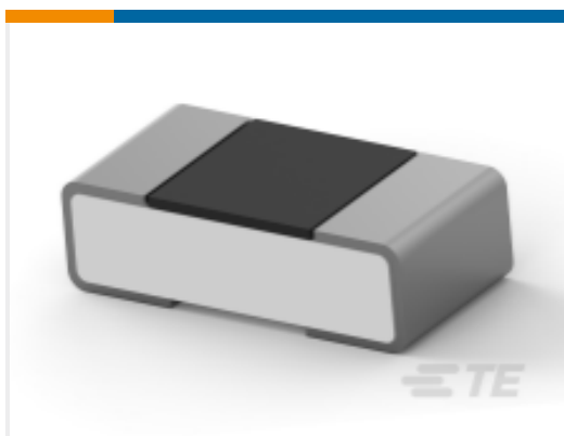
TE Model / Part #4-2176364-9 RQ 0402 14K7 0.1% 10PPM 5K RL
