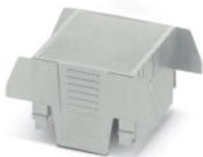
DIN rail housing, Upper part, connection opening on both sides, width: 52.6 mm, height: 74.65 mm, Depth: 36.95 mm, color: light gray (7035)
