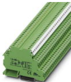
Power solid-state relay terminal block, input: 24 V DC, output: 10 - 253 V AC/800 mA, terminal block width: 6.2 mm
