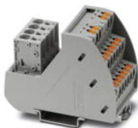
VARIOFACE module, with two equipotential busbars (P1, P2) for potential distribution, for mounting on NS 35 rails. Module width: 41.9 mm
