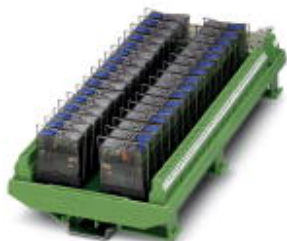
VARIOFACE output module, with 32 miniature relays, 1 PDT with detectable manual operation each, plugged, for 24 V DC (incl. relay)
