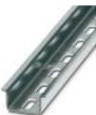
DIN rail perforated, Standard profile, width: 35 mm, height: 15 mm, similar to EN 60715, material: Steel, Galvanized, white passivated, length: 2000 mm, color: silver
