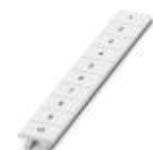
Zack marker strip, Strip, white, labeled, can be labeled with: CMS-P1-PLOTTER, Printed vertically: consecutive numbers 1 ... 10, 11 ... 20, etc. up to 91 ... 100, mounting type: snap into tall marker groove, for terminal block width: 8.2 mm, lettering field size: 10.5 x 8.15 mm
