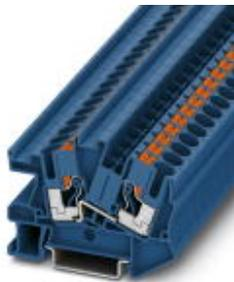
Installation terminal block, Push-in connection, cross section: 0.5 mm<sup>2</sup> - 10 mm<sup>2</sup>, AWG: 20 - 8, width: 8.2 mm, color: blue, mounting type: NS 35/7,5, NS 35/15
