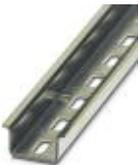
DIN rail perforated, Standard profile, width: 35 mm, height: 15 mm, similar to EN 60715, material: Steel, galvanized, passivated with a thick layer, length: 2000 mm, color: silver
