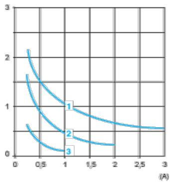
DC- Control of electromagnets ( $L/R \leq 2 \times (U_e \times I_e)$  in ms, with  $U_e$ : rated operating voltage and  $I_e$ : rated operating current)
