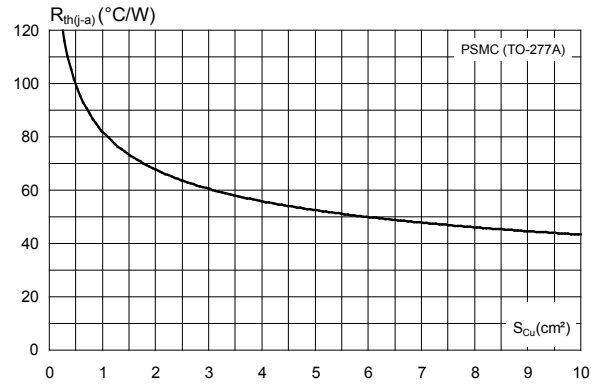
Figure 11. Thermal resistance junction to ambient versus copper surface under tab (typical values, epoxy printed board FR4, e_{Cu} = 35 \mu m ) (PSMC (TO-277A))
