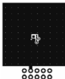
a. 80^\circ\text{C}/\text{W} when mounted on a 1 in 2 pad of 2 oz copper
