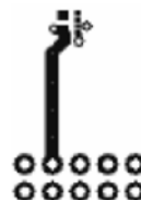
b. 165^\circ\text{C}/\text{W} when mounted on a minimum pad of 2 oz copper
