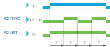
Function Di - Symmetrical flashing (ON Start)
