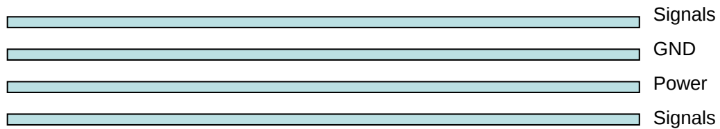
Figure 29: Typical 4-layer PCB construction
