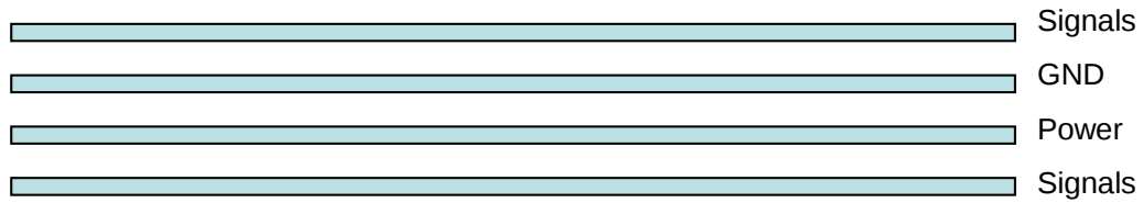
Figure 17: Typical 4-layer PCB construction
