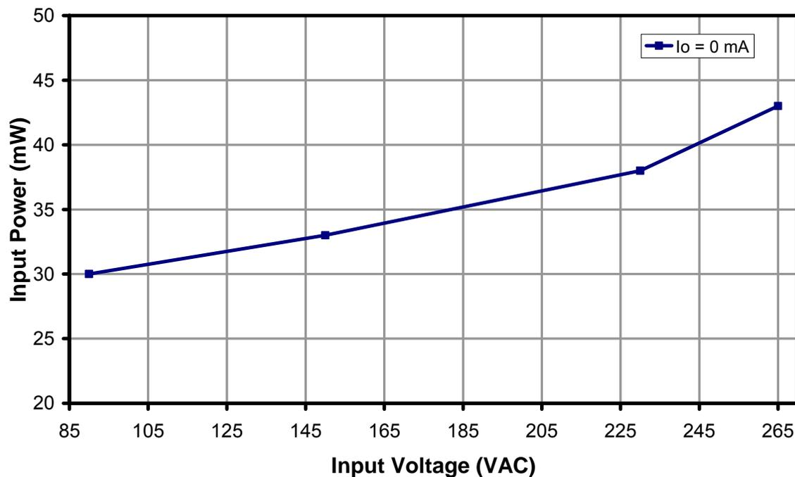
Figure 7 – No-load Power Consumption, Room Temperature.
