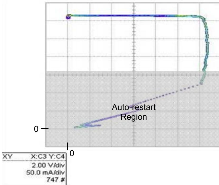
Figure 9 – CC/CV Curve at 120 VAC Input, Room Temperature.
