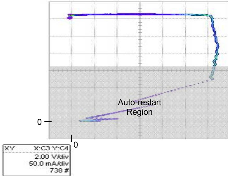
Figure 10 – CC/CV Curve at 230 VAC Input, Room Temperature.
