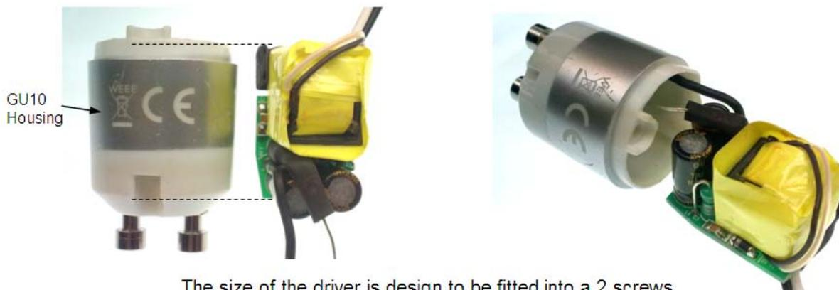
The size of the driver is design to be fitted into a 2 screws holes GU10 lamp housing
