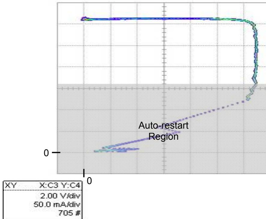
Figure 11 – CC/CV Curve at 265 VAC Input, Room Temperature.
