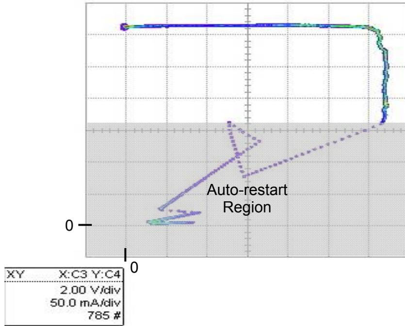
Figure 8 – CC/CV Curve at 90 VAC Input, Room Temperature.
