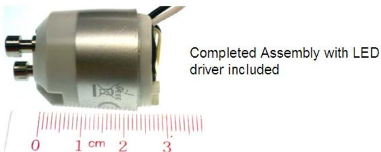
Figure 2 – Assembled Driver Inside GU10 Base.
