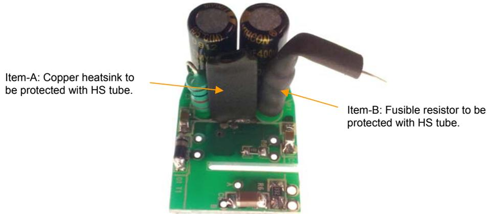
**Item-A: Protect copper heatsink with heat shrinkable tube**
