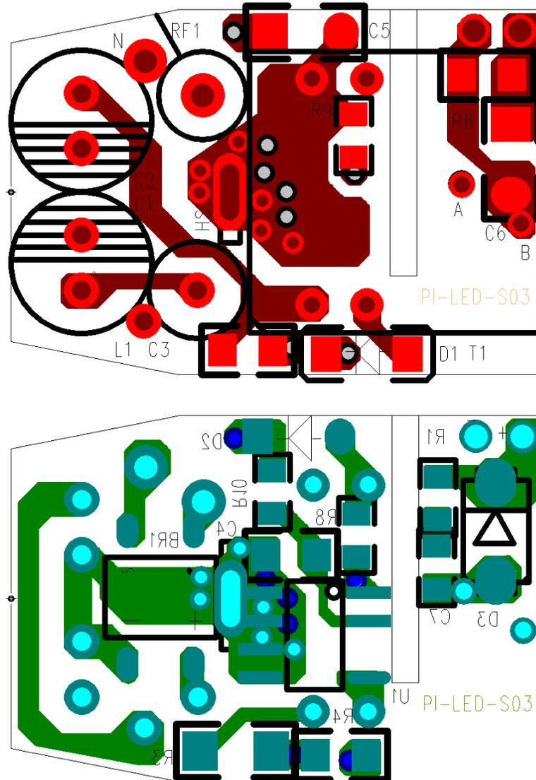
**Figure 4** – Printed Circuit Layout (Designed to Fit Inside GU10 Lamp Form Factor).
