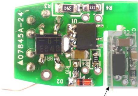
Note : the assembly has a heat shrinkable tube to cover & protect the entire secondary circuits to meet ESD and Hipot test requirement
