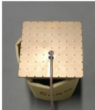
Ground above antenna
