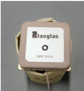
Ground under antenna
