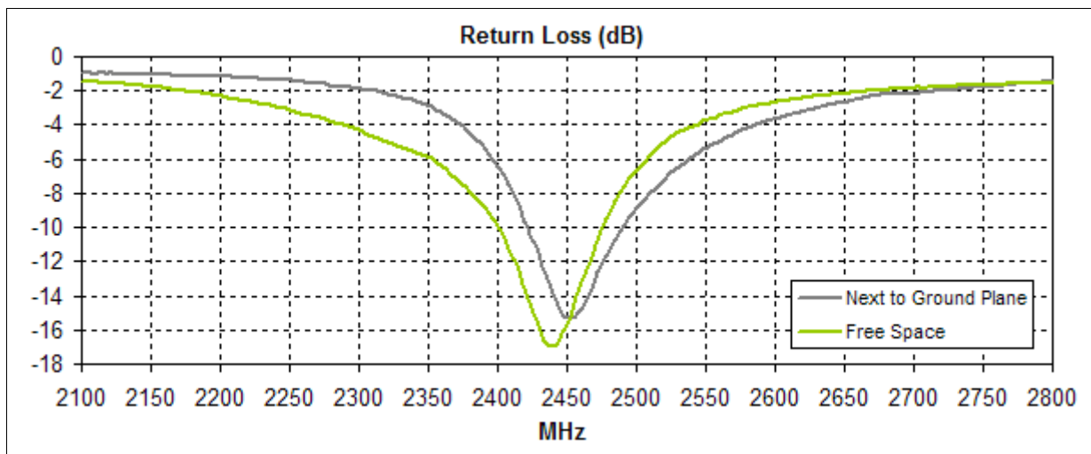
Figure 3. Return Loss for the FXP72 Antenna.
