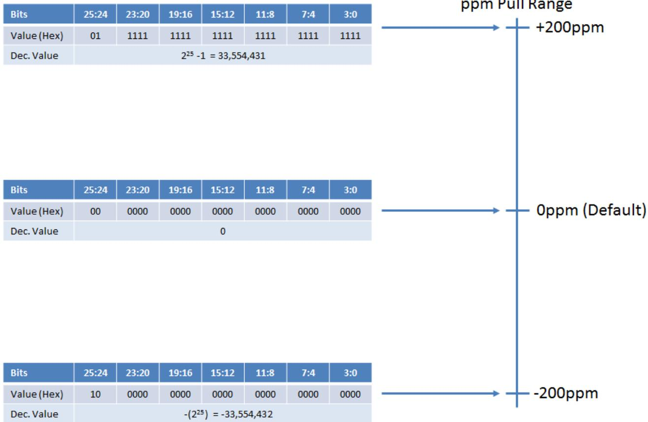
**Figure 29. Pull range and Frequency Control Word**
