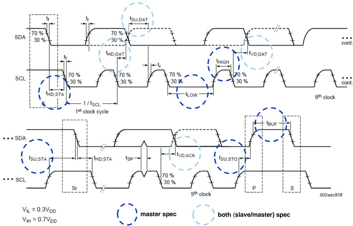
Figure 35. I<sup>2</sup>C Timing Diagram
