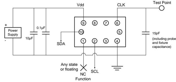
**Figure 12. LVMOS Test Circuit (I<sup>2</sup>C Control)**
