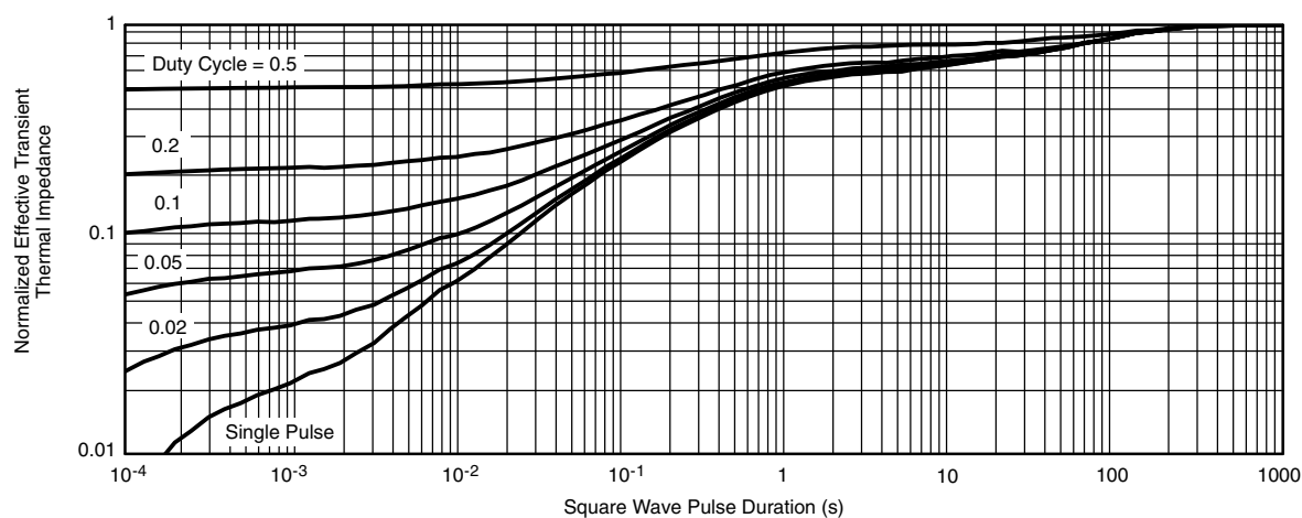
Normalized Thermal Transient Impedance, Junction-to-Ambient
