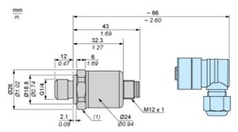
(1) SW24 tightening torque ≤ 25 N.m / 221 lb-in
