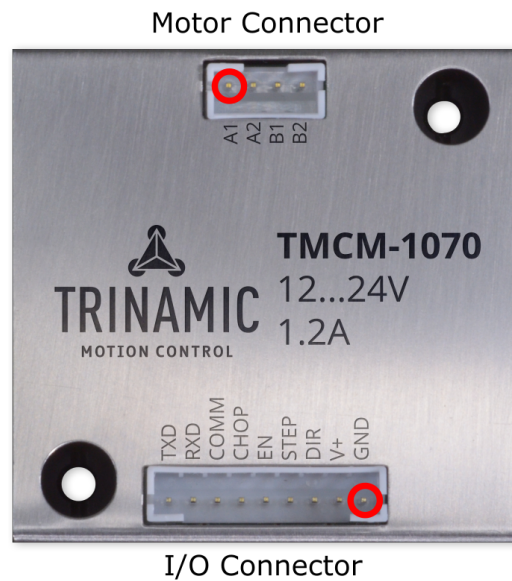
Figure 7: TMC-1070 connectors (pin 1 highlighted in red)
