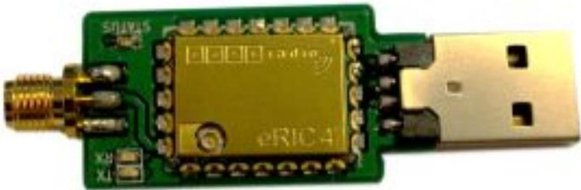
The eRIC4-USB dongle is fully USB compatible, offering customers a simple, ready-to-use and flexible modem for enabling any USB host device with 433MHz ISM radio communications.
