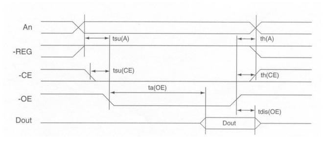
Figure 4. Common Memory Read Timing Diagram
