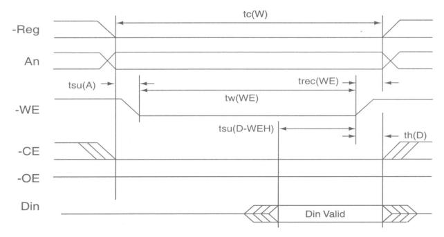
Figure 3. Configuration Register (Attribute Memory) Write Timing Diagram
