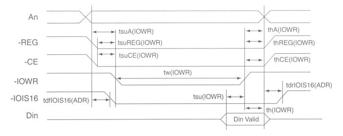
Figure 7. I/O Write Timing Diagram
