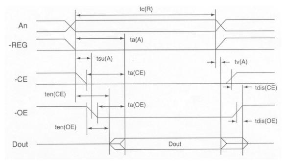
Figure 2. Attribute Memory Read Timing Diagram
