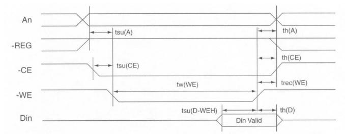
**Figure 5. Common Memory Write Timing Diagram**
