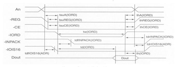
Figure 6. I/O read Timing Diagram
