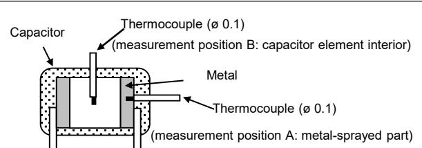
When a capacitor is sent through a high-temperature atmosphere after being subjected to the (flow) soldering process, check the mounting temperature including the temperature of the capacitor in the high-temperature atmosphere.
