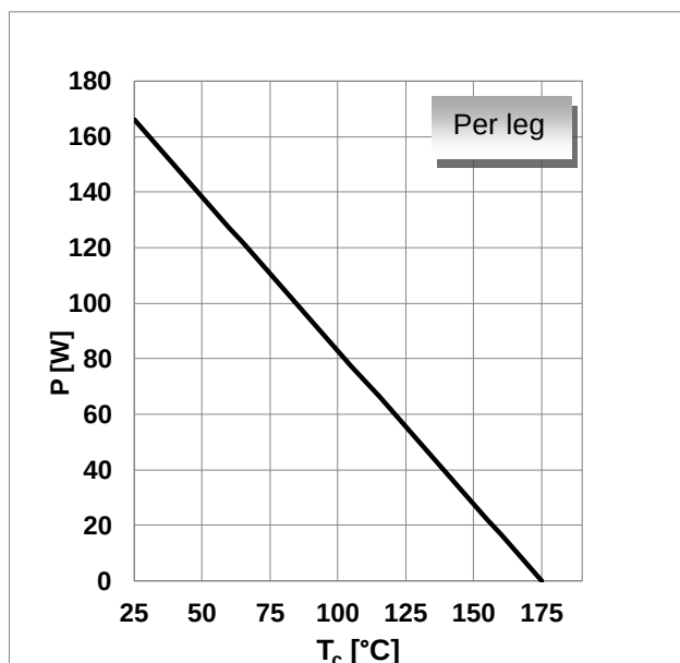
Figure 1. Power dissipation per leg as function of case temperature, P_{\text{tot}} = f(T_c) , R_{\text{th(j-c),max}}
