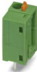
PCB terminal block, nominal current: 15 A, nom. voltage: 320 V, pitch: 7.62 mm, number of positions: 1, connection method: Push-in spring connection, mounting: Wave soldering, conductor/PCB connection direction: 90 °, color: green. End terminal block for terminating custom-grouped blocks.
