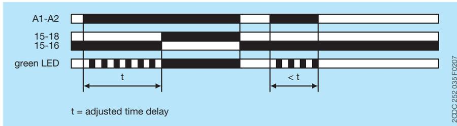
■ OFF-delay with auxiliary voltage
