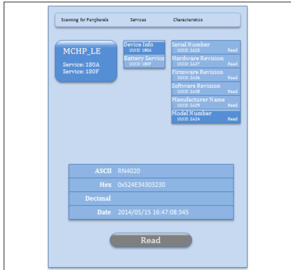
FIGURE 3-2: READING THE MODEL NUMBER STRING FROM THE DEVICE INFORMATION SERVICE
