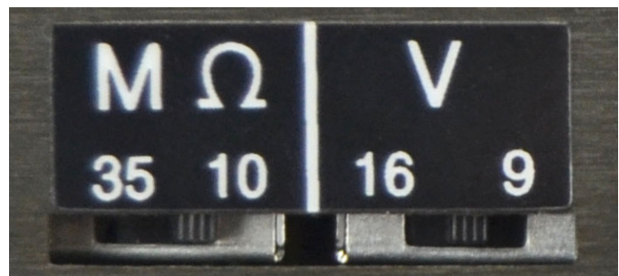
Figure 4. Operator test limit and test voltage switches located on the right-side of the monitor
