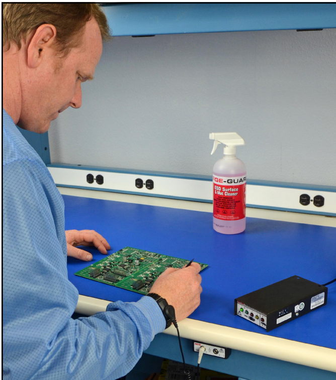
Figure 9. Using the 724 Workstation Monitor
