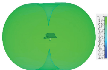
Typical 3D Radiation Patterns - Cell / LTE Elements 1 & 2
