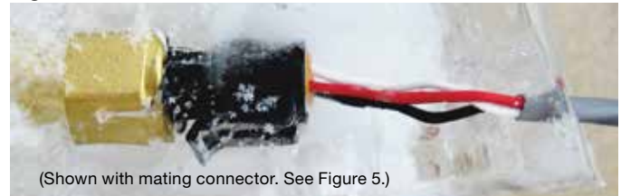
Figure 2. PX3 Series External Freeze/Thaw Resistance
