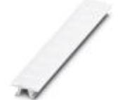
Zack marker strip, can be ordered: Strip, white, labeled according to customer specifications, Mounting type: Snap into tall marker groove, for terminal block width: 6.2 mm, Lettering field: 6.15 x 10.5 mm
