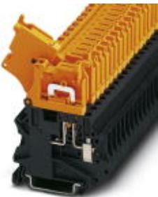
Disconnect terminal block, With test socket screws for insertion of test plugs, Connection type: Screw connection, Cross section: 0.14 mm<sup>2</sup> - 6 mm<sup>2</sup>, AWG: 26 - 10, Nominal current: 20 A, Nominal voltage: 500 V, Length: 57.8 mm, Width: 6.2 mm, Color: black/orange, Assembly: NS 35/7,5, NS 35/15
