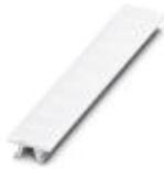
Marker for terminal blocks, Strip, white, labeled, can be labeled with: CMS-P1-PLOTTER, Horizontal: L1, L2, L3, N, PE, L1, L2, L3, N, PE, Mounting type: Snap into tall marker groove, for terminal block width: 6.2 mm, Lettering field: 6.15 x 10.5 mm
