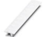
Zack marker strip, Strip, white, labeled, can be labeled with: CMS-P1-PLOTTER, Printed vertically: Consecutive numbers 1 - 10, 11 - 20, etc. up to 491 - 500, Mounting type: Snap into tall marker groove, for terminal block width: 6.2 mm, Lettering field: 6.15 x 10.5 mm
