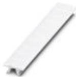
Zack marker strip, Strip, white, labeled, can be labeled with: CMS-P1-PLOTTER, Printed horizontally: Identical numbers 1 or 2, etc. up to 100, Mounting type: Snap into tall marker groove, for terminal block width: 6.2 mm, Lettering field: 6.15 x 10.5 mm
