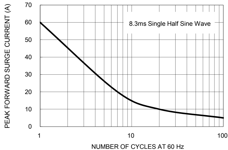
FIG. 3 MAXIMUM NON-REPETITIVE PEAK FORWARD SURGE CURRENT
