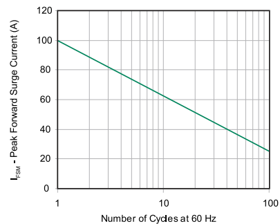
Figure 6 - Maximum Non-Repetitive Peak Forward Surge Current Uni-Directional Only
