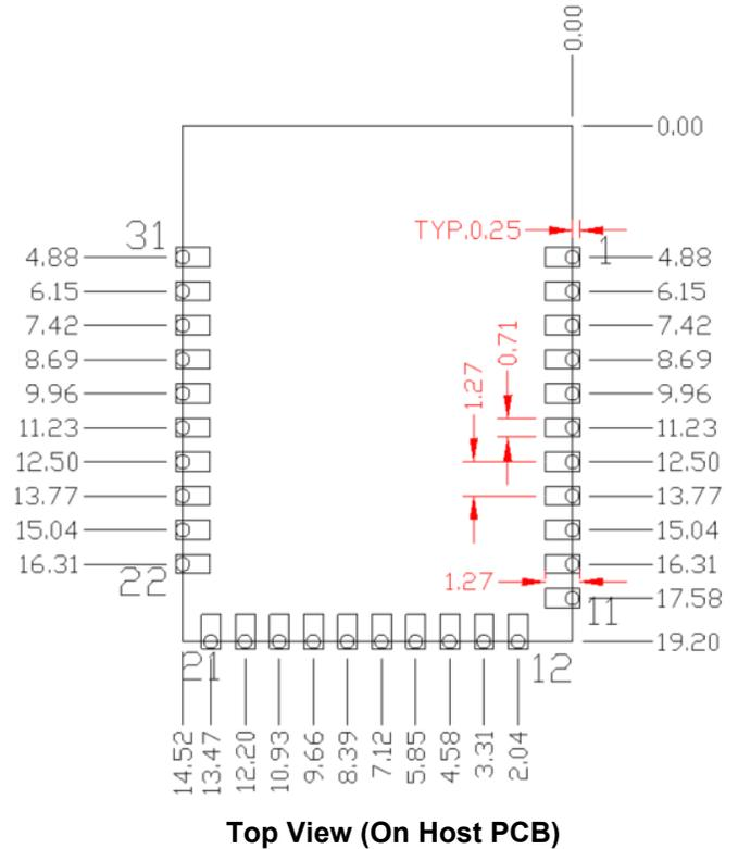
Table 3 provides the center location for each solder pad on the CYBLE-2120XX-X0. All dimensions reference the to the center of the solder pad. Refer to Figure 6 for the location of each module solder pad.
