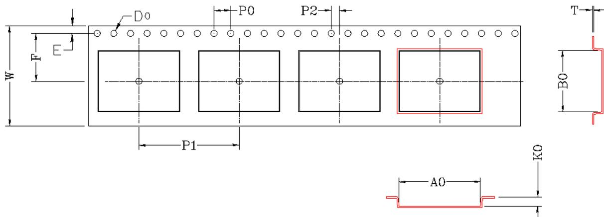
[Figure 11](#) details the orientation of the CYBLE-2120XX-X0 in the tape as well as the direction for unreeling.
