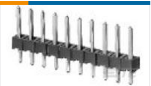
TE Part #9-146280-0 40 MODII HDR SRST B/A .100CL
