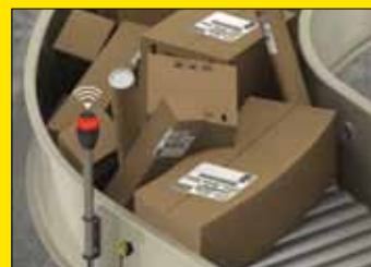
Manufacturing Line Blockage Indication A red, audible domed light alerts operators of congestion due to a box pile up.
