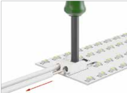
Inserting/removing fine-stranded conductors by lightly depressing the push-button (e.g., using the optional 206-860 Operating Tool).
