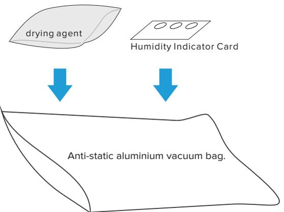
The vacuum bag is placed inside the box and a Model Name Label stuck on the front-side of each box.
