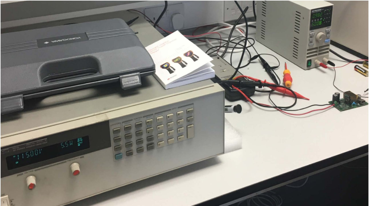
Figure 10 Test Bench Showing Input and Output Power (91.05 % Efficiency)
