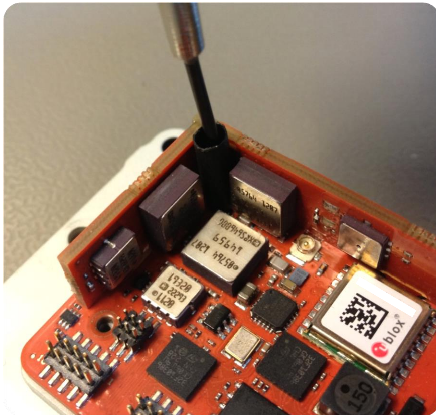
Figure 11: Using a heat shrink tube to position the mounting screws
